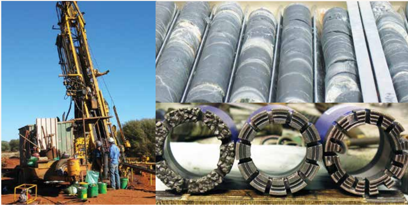
After identifying a key location for further exploration, a diamond drill rig is brought in to bore the target mineralization zones. The hollow drill tips (lower right) allow removal of core samples (upper right) that are withdrawn from depths that can extend hundreds of feet below surface.
